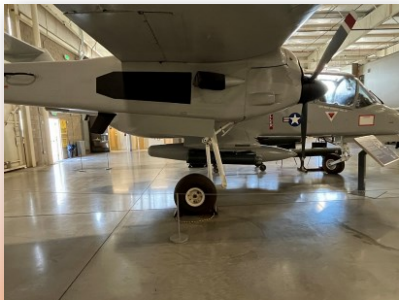
Side on view of the right main landing gear with its trailing link design.
