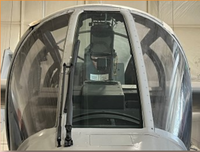
A couple views of the canopy showing the windshield wiper on the center of the windscreen.
