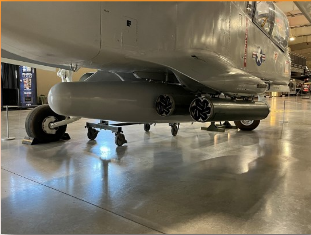
View from the aft right side showing the back of the right side rocket launchers and the center-line drop tank.
