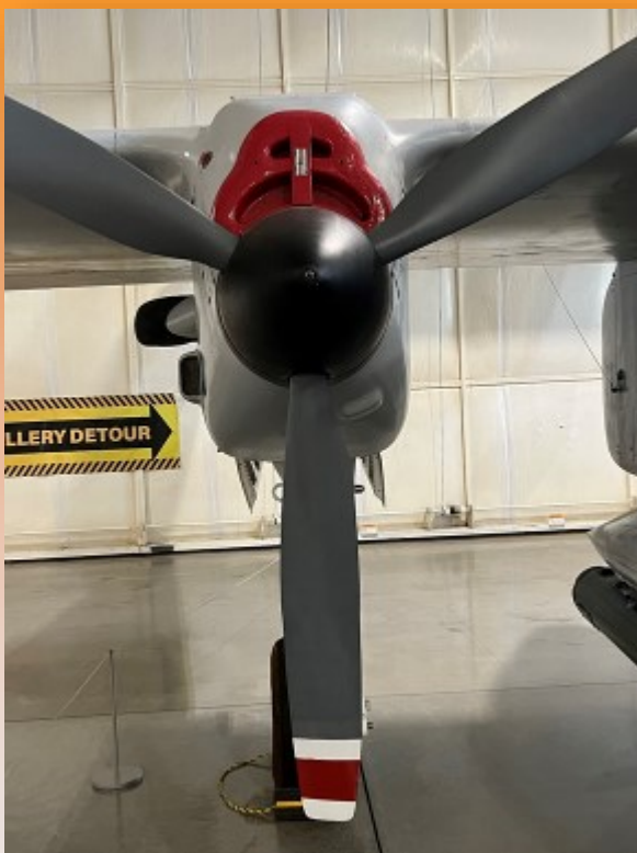
Head on view of the right boom and engine. The engine has red intake covers installed as can be seen above the propeller spinner. Also note the engine exhaust on the outboard side.
