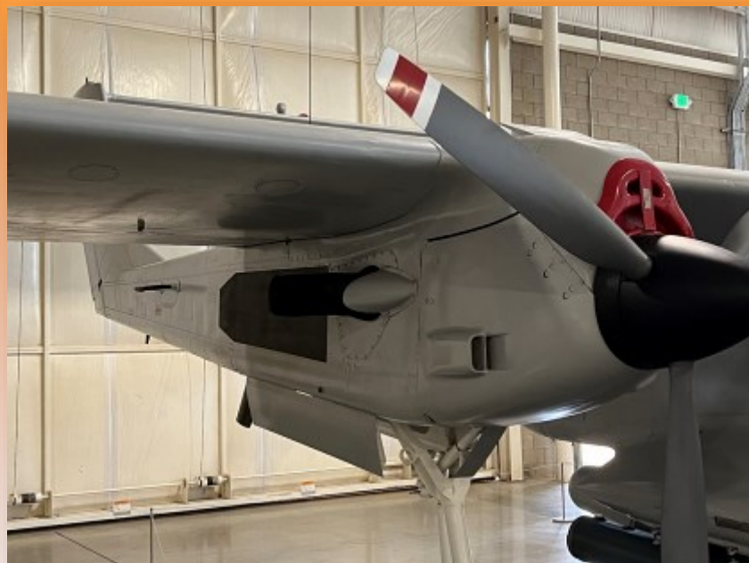
A different view of the outboard side of the right boom showing the engine exhaust and an air intake as well as the top of the right main landing gear strut.
