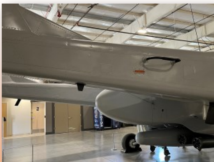
Right side aft section showing a towel rack style antenna above an orange light similar to those on the nose.
