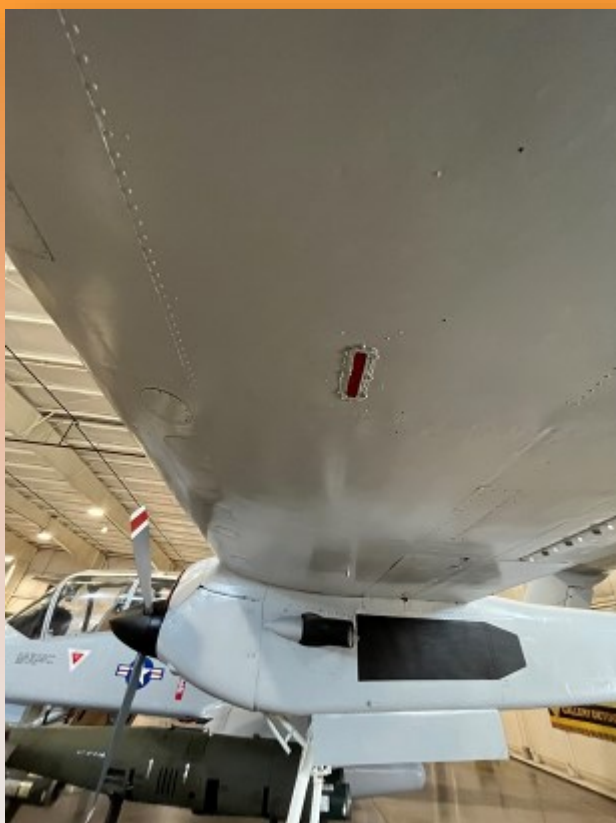
The left wing has a corresponding red light, most likely part of the navigation light system as seen in the following photo.
