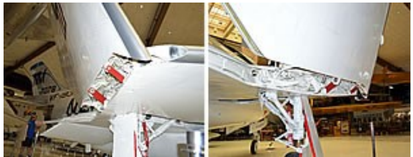
Starboard wing fold line details.
