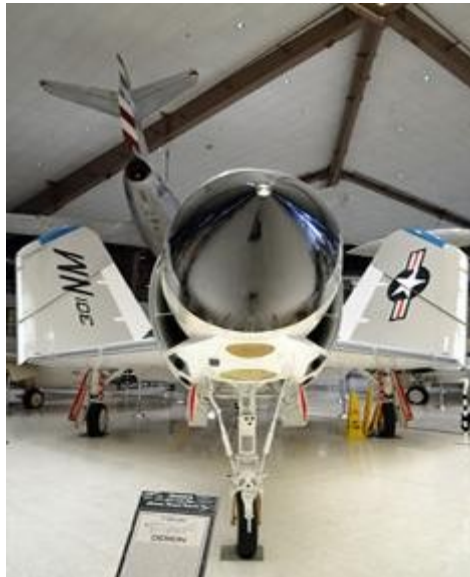
Head on view showing the layout of the four 20mm cannon ports, the air intakes, and the nose gear geometry. Also note the angle of the wing fold line.
