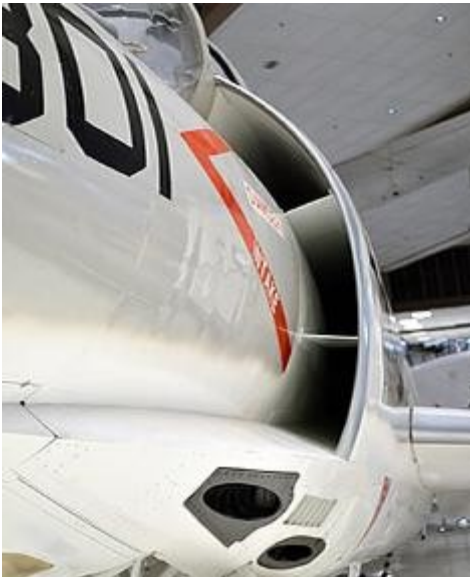
The port side cannon ports can be seen under the port air intake.
