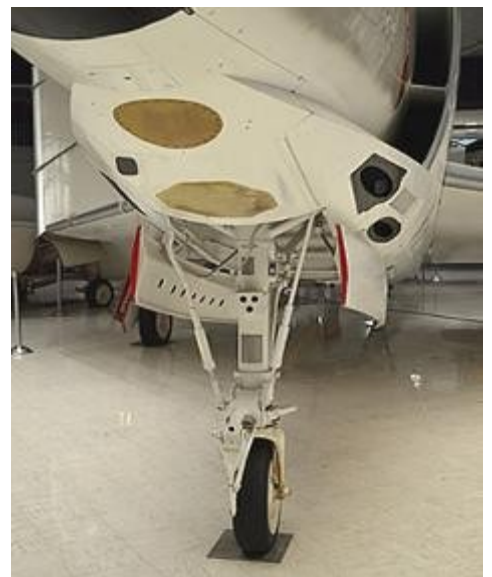
Head on view showing the layout of the four 20mm cannon ports, the air intakes, and the nose gear geometry. Also note the angle of the wing fold line.
