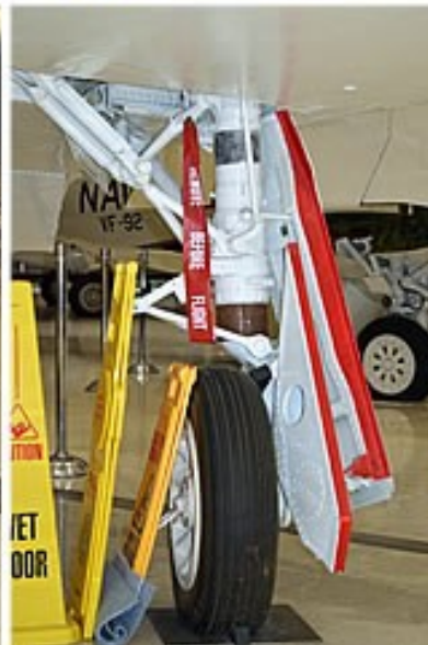
Details of the port side main landing gear and wing fold.
