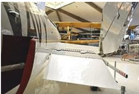
Starboard wing flap looking forward. Interesting items include what appears to be a perforated spoiler on the top of the wing, a red striped fuel vent outboard of the flap, and a partially open speed brake on the fuselage.
