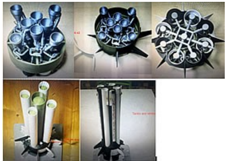
Figures 5, 6, 7, 8 and 9: Stages of assembly of Stage 1
